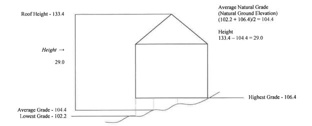
Natural Ground Elevation or Natural Grade Elevation is defined as the elevation of the existing ground surface prior to any disturbance of the site resulting from construction of the proposed improvements.
